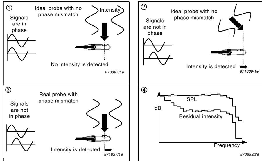
1. A sound wave is incident on a probe axis at  $90^\circ$ . There is no flow of acoustic energy along the probe axis. The signals from the microphones are in phase and no intensity is detected.
